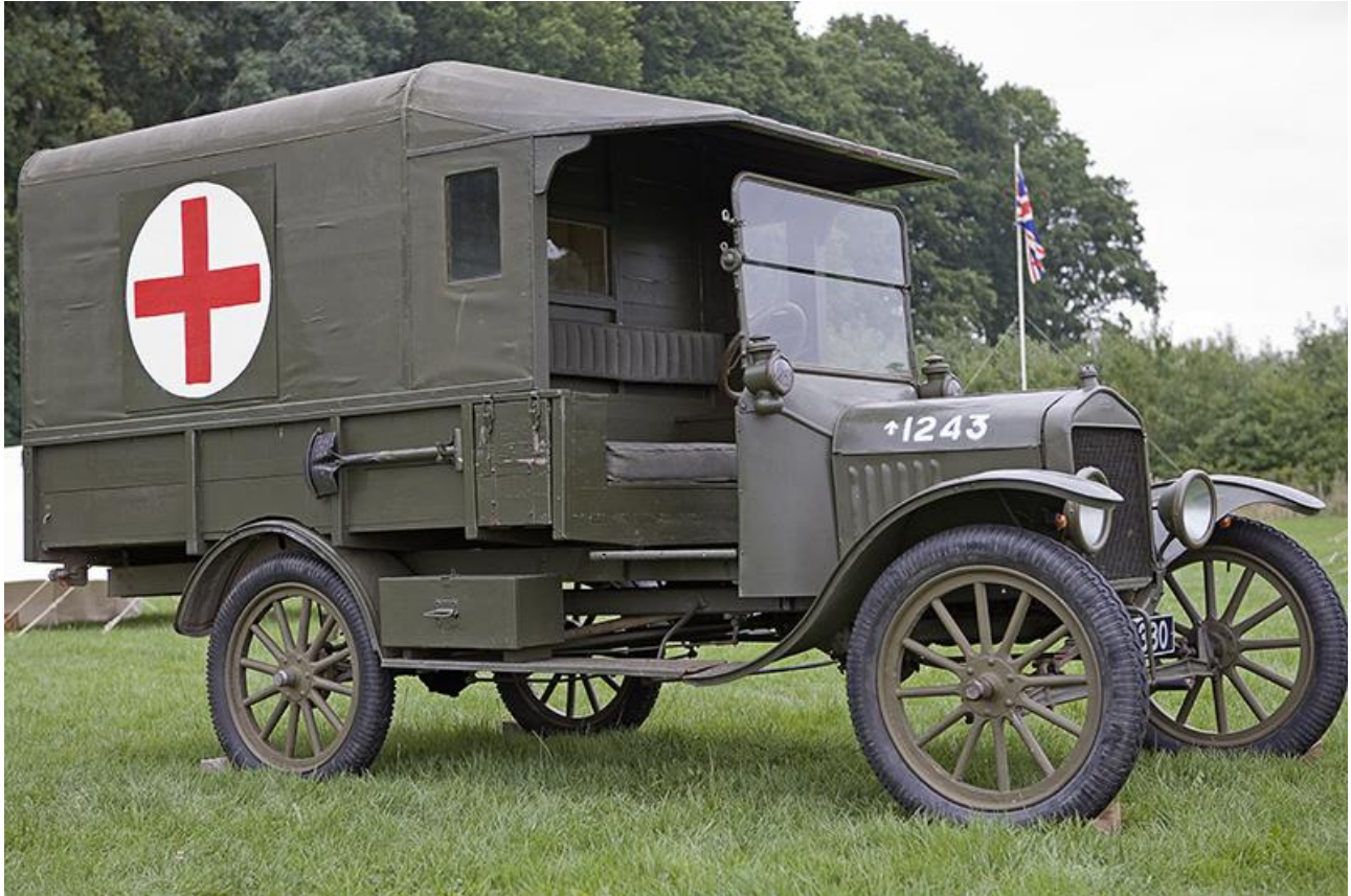
Ford 1916 Model T Field Ambulance. This canvas on wood frame model was used extensively by the British & French as well as the American Expeditionary Force in World War I . Its top speed was 45 mph (72 km/h), produced by a 4-cylinder water-cooled engine.
