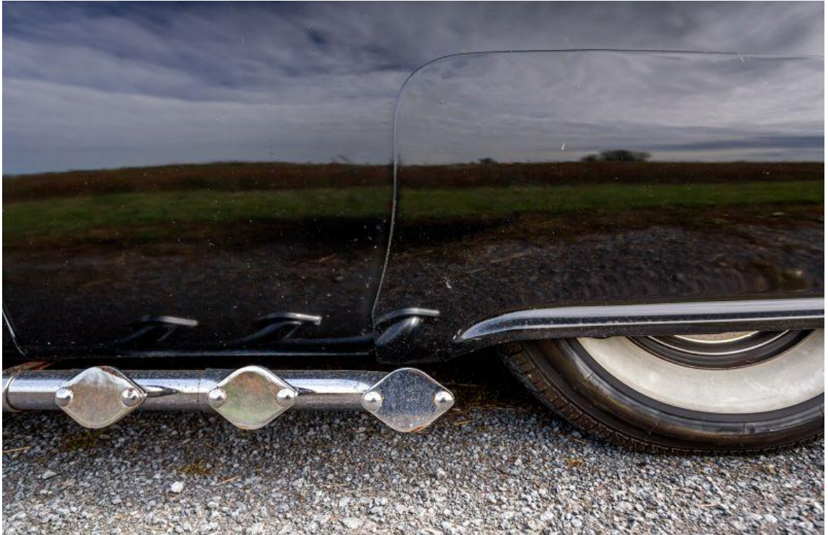
A set of triple-outlet chrome lake pipes throwback to 1950s' kustom cars.
