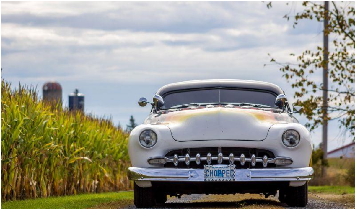
Adding a different grille with additional teeth was another customizing trick from the 1940s and '50s.
