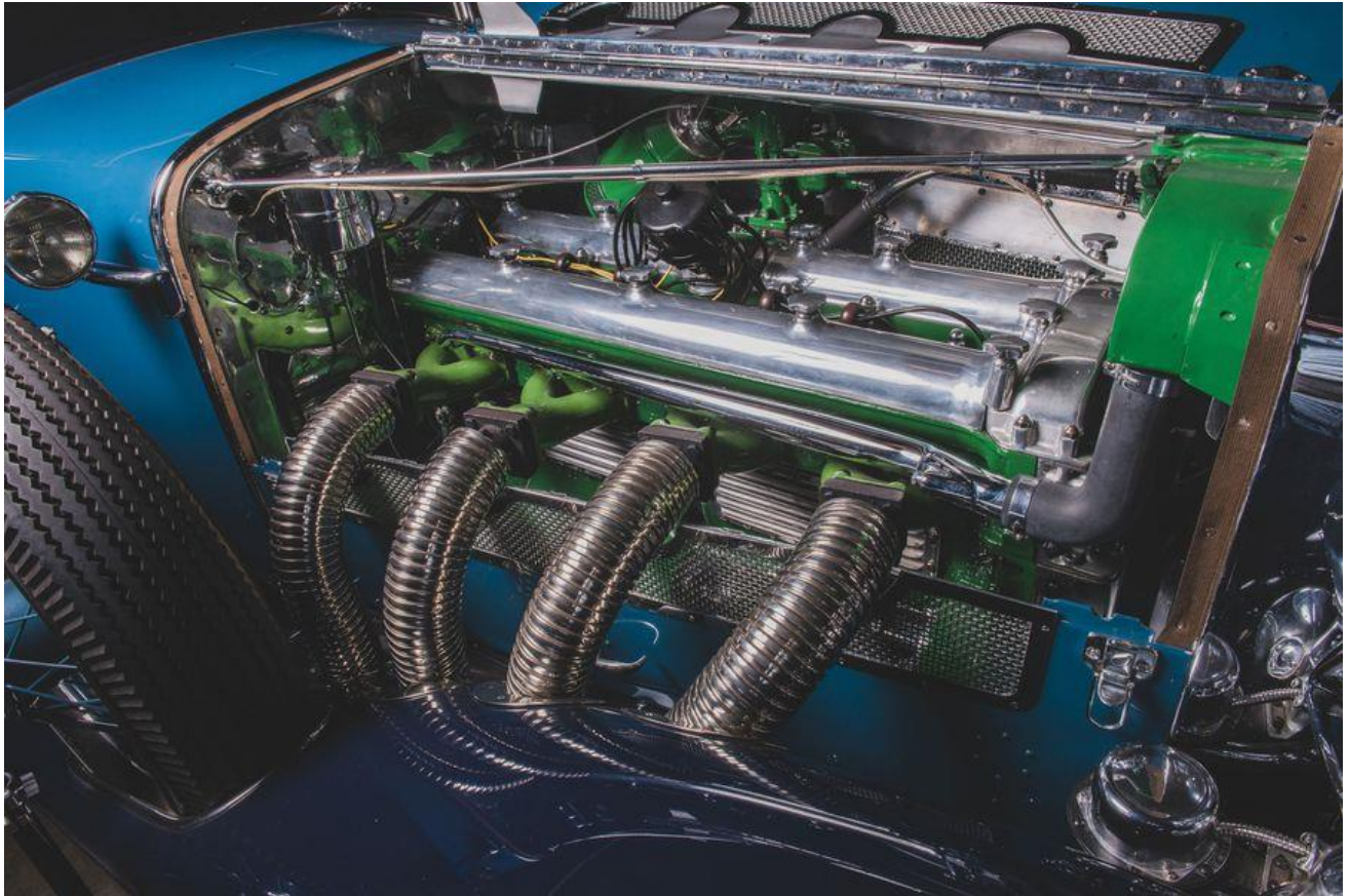
Duesenberg Model J DOHC straight-eight. Photo by Darin Schnabel, via RM Sotheby's.
