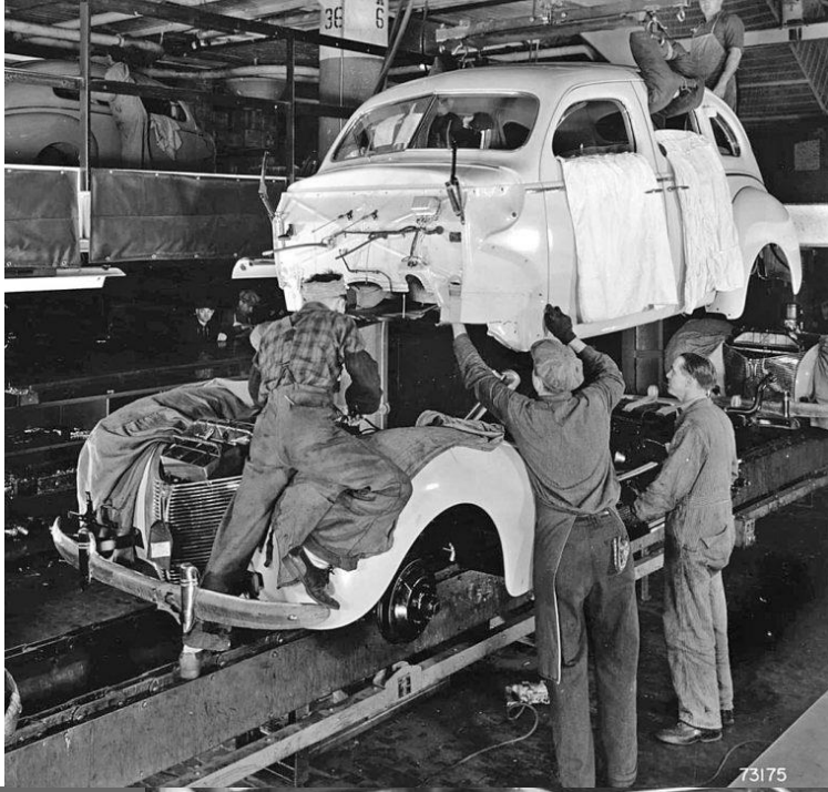
1940 Mercury body drop station on the assembly line.
