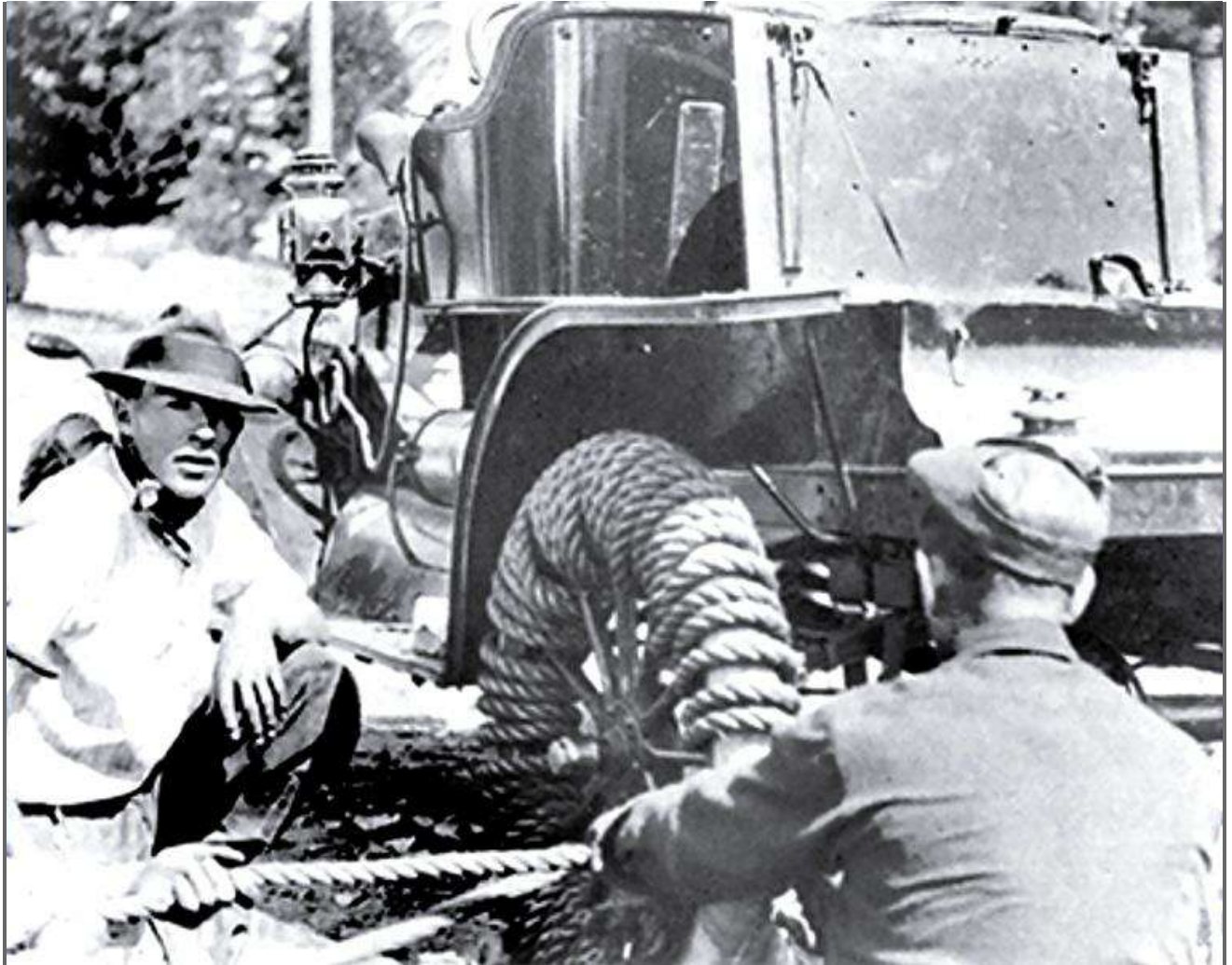
Rope was wound around the rear tires and wheels for traction during the trip.
