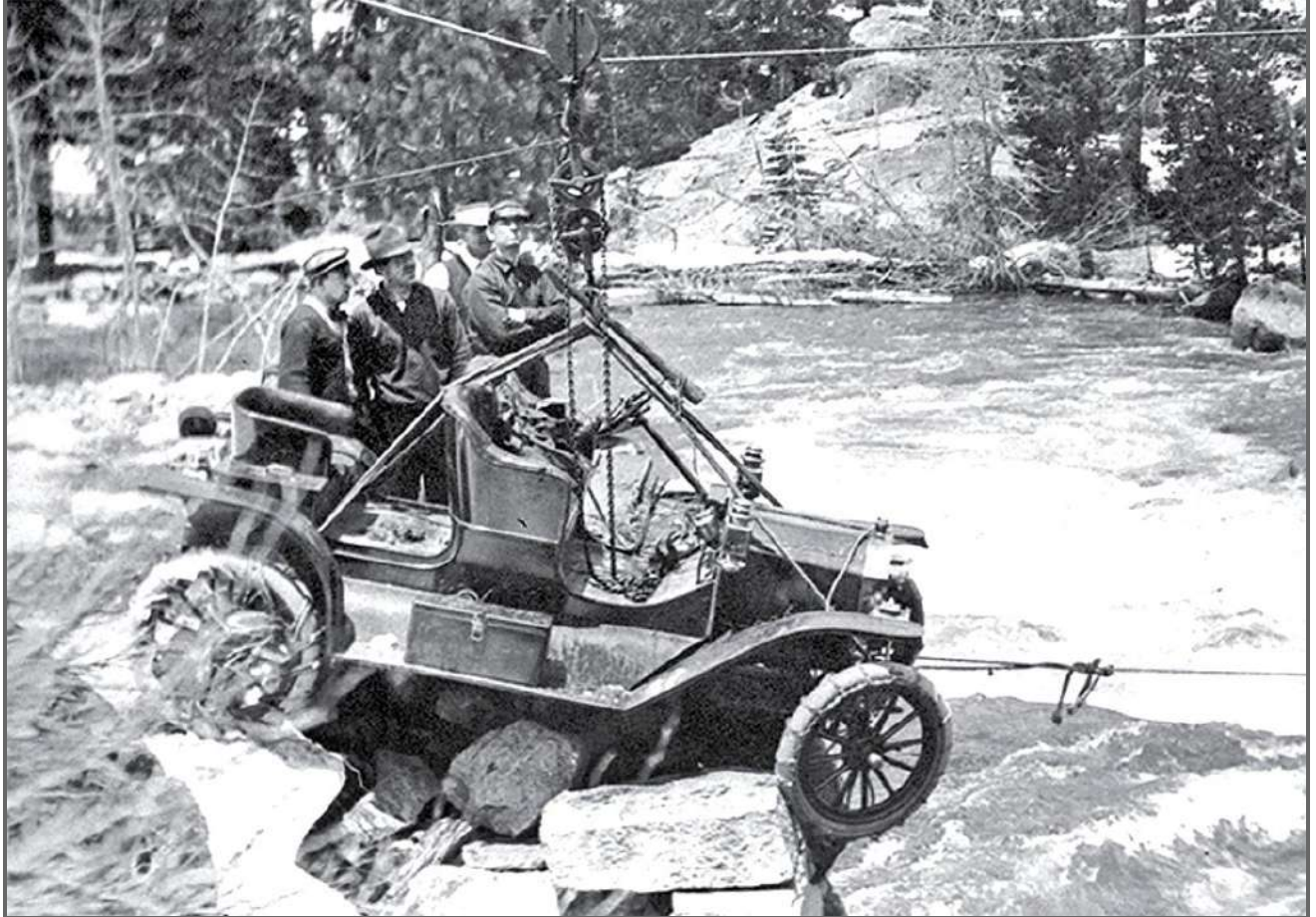
After discovering the bridge over the Yuba river had washed away the crew moved the Ford over the river by using a cable, pulley, chain falls, and rope.
