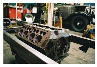
The first of the Ford L-head (flathead) V8 engines left the factory on March 9, 1932. This engine used a 90degree block, with the valves located next to the pistons, pointed upwards. The heads are not truly flat, having four spade-shaped combustion chambers to accommodate the motion of the valves. The geardriven cam was located in the engine block above the crankshaft and between the cylinder banks, driving solid lifters that acted directly on the valves. There
