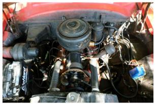
For 1939, Mercury added a new variant of the Ford flathead V8 design. The new engine was larger, displacing 239.4 cubic inches by virtue of a longer 3.1875-inch stroke. At a stock compression ratio of 6.3:1, the new Model 99A offered 95 horsepower. V8 production passed the 6-million-unit mark during this year.
