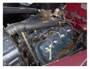
In the history of automotive engines, it's impossible to overstate the importance of the V8 design. By dividing the eight cylinders into two banks of four, engineers achieved a powerful, yet compact unit that could fit into the vast majority of engine bays also sized to fit four or six-cylinder engines.
