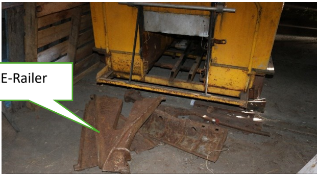
This unique item is called a “RE-RAILER” it is used to get rail cars & engines back on the rails after a derailment. Cars were pulled back on the tracks guided in place. Ingenious for sure.
