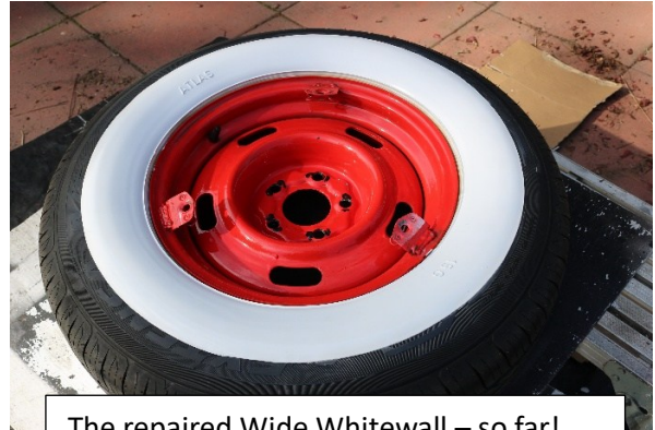
The repaired Wide Whitewall – so far!
