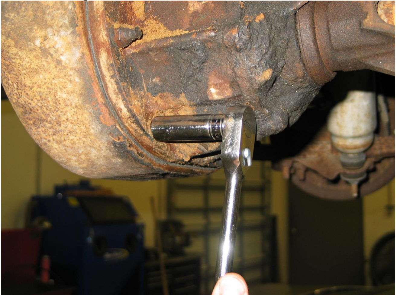
Checking A Ford Axle With a Deep Socket To Confirm If It Is a 8-Inch or 9-Inch
